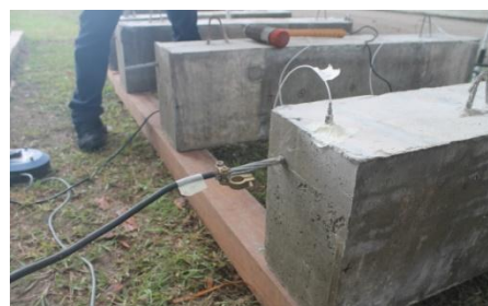
Fig. 4: High Electric Current Routed into Concrete
