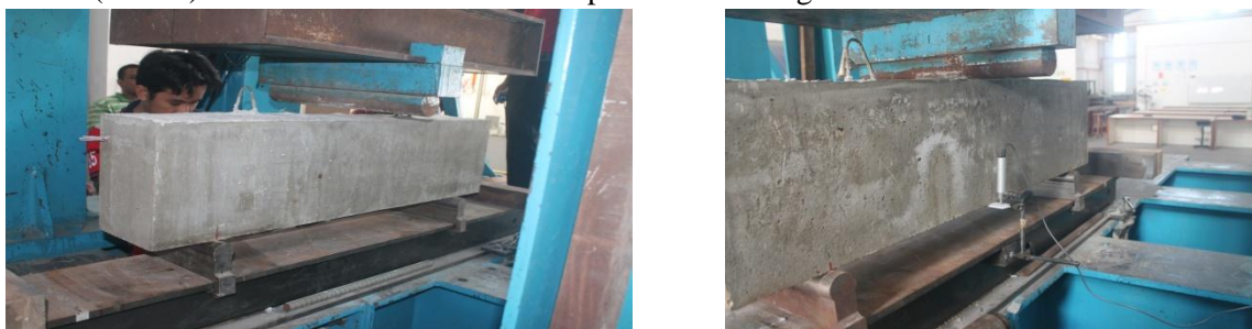
Fig. 5: Flexural Testing Arrangement and LVDT
