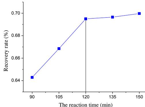
Fig. 5: The relationship between reaction time and the recovery rate of PbS
