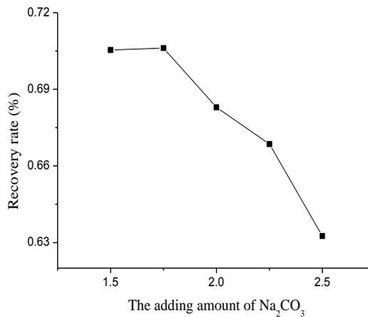
Fig. 3: The relationship between addition of Na<sub>2</sub>CO<sub>3</sub> and the recovery rate of PbS.
