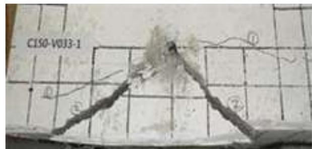
Fig. 4: Failure shape of the anchor specimen in the SFRC with the fiber volume fraction of 0.33%
