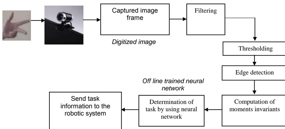
Fig.1 The block scheme of the designed vision based control of a robotic system.
