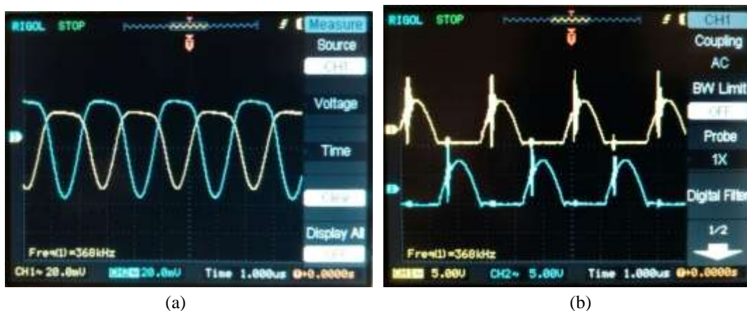
Fig. 7: (a) gate to ground signals (b) Drain to ground signals
